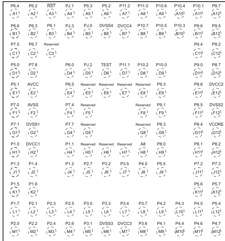
Figure 4-2. 113-Pin ZQW Package (Top View)
