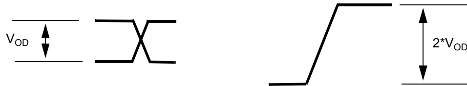
Figure 19 - Differential Output Voltage Parameter
