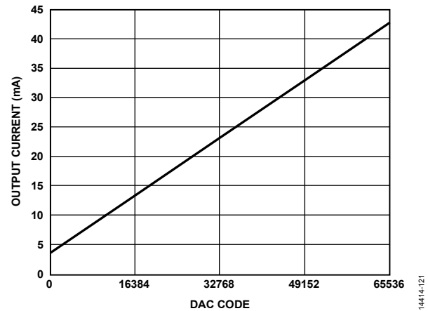
Figure 138. Gain Curve for ANA_FULL_SCALE_CURRENT[9:0] = 1023, DAC Offset = 3.8 mA
