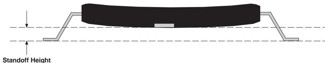
Figure 7-1. Standoff Height Measurement on 144-Pin RFP Package
