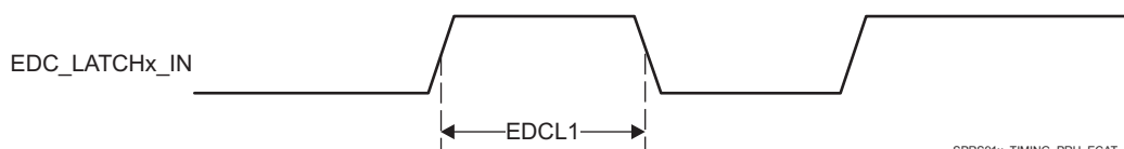
Figure 5-69. PRU-ICSS ECAT LATCHx_IN Timing
