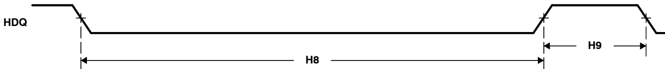
Figure 5–39. HDQ/1-Wire Break (Reset) Timing
