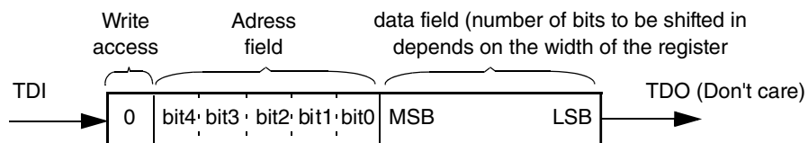
Figure 4-29. TDI/TDO on write access
