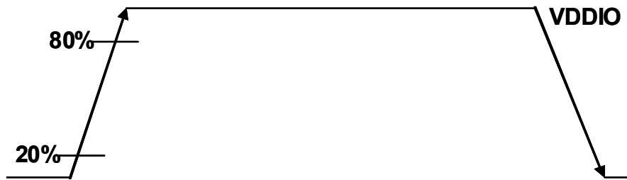
Figure 4. Output Pad Transition Waveform
